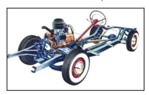
The numerous improvements included a new box-section frame, redesigned front and rear suspension, tubeless tires, and a 12-volt ignition system—a necessary upgrade to support the high-compression 265 CID V8. As we know, it was the exciting new V8 that came to dominate the Chevrolet story for 1955. But actually, there were a number of interesting developments that are worth a closer look.
